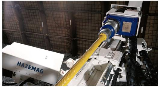
**Drilling/bolting device with HDR 1**
